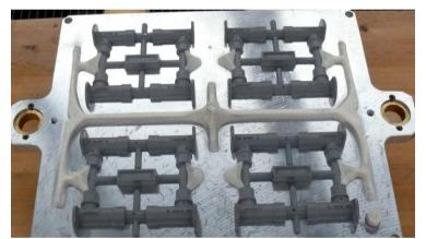
Casting mould in process (left), Instead of usual release agents, casting moulds coated with **long-lasting paint RK CCS**. The ceramic coating is resistant to temperature, for metal casting.
