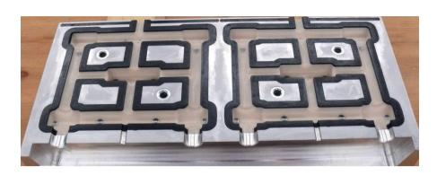
Instead of the usual release agents, casting moulds coated with **long-lasting RK CCS paint**. Dry layer thickness approx. 2-3  $\mu$ m.
